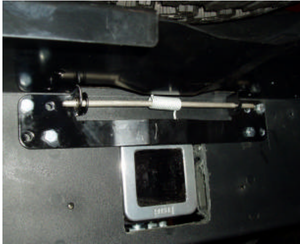
Fig 9: Shows number plate bracket on vehicle, when not towing.
