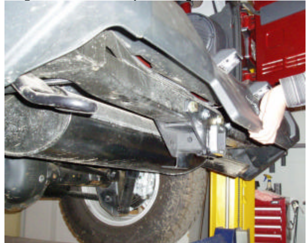
Fig 6: Shows bumper being flexed out.
