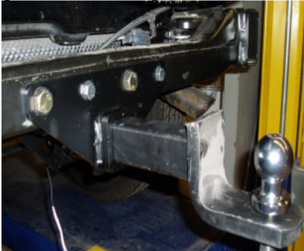
Fig 7: Shows towbar being mounted on the vehicle.
