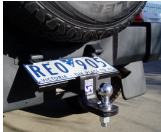
Fig 10: Shows number plate bracket being flipped up while towing.
