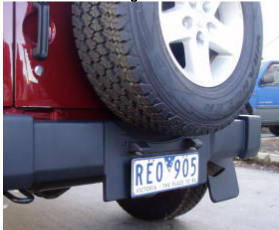
Fig 9: Shows number plate bracket on vehicle, when not towing.
