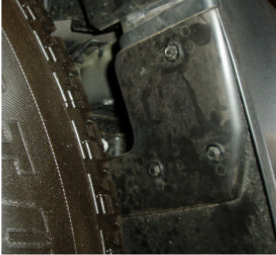
Fig 3: Remove 3 screws on Mudflap shown.
