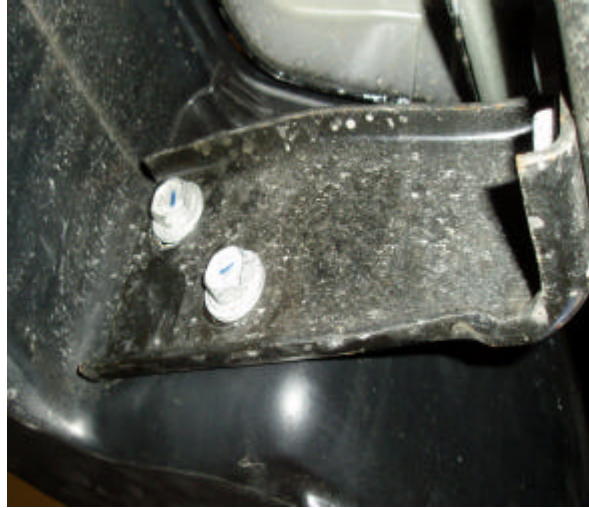
Fig 4: M10 bolts behind mudguard
