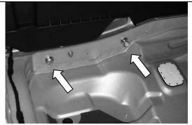
9. Locate chassis inserts to vehicle. Loosely secure both forward mounts using M10x1.5x35 Bolts, M10 Spring Washer, M10 Flat Washers.
