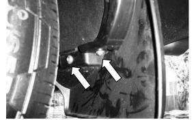
Remove the 3 scrivets and 2 bolts (or 5 scrivets on vehicles without mudguard) holding the mudflaps to the bumper. (Both RH and LH side)
