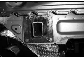
Loosely secure the chassis inserts to the rear panel on the vehicle using M10x1.5x35 Bolts, M10 Spring Washer, M10 Flat Washers and M10 Nuts.
