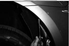
3. Pull back wheel arch trim and remove the forward most bolt holding the bumper to the vehicle.
