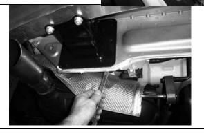
8. Remove the eight nuts holding the rear impact beam to the vehicle.
