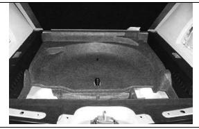
5. From inside the vehicle, remove the spare tyre and the jack assembly from rear tyre well.
