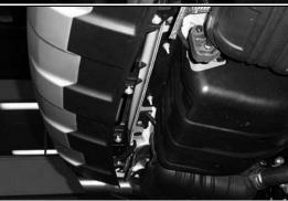
4. Remove the four bolts holding the bottom of the bumper to the vehicle.
