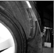
2. If mudflap is fitted, remove the forward-most bolt holding the mudflap bracket and wheel arch trim to the vehicle.
