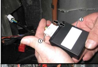
14. Apply double sided tape to the ECU (1) and adhere it to the vehicle sheet metal on the RHS of the luggage compartment.
