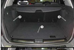
3. Remove the rear trim (1) by first removing the two fasteners (2).
