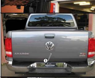
7. Remove the LHS tail light (1) by first removing the two T30 torx bolts (2).
