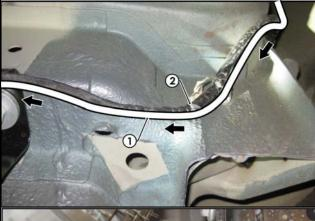
11. Connect 24-way waterproof ECU (04835) connector (1) to the ECU (2).
