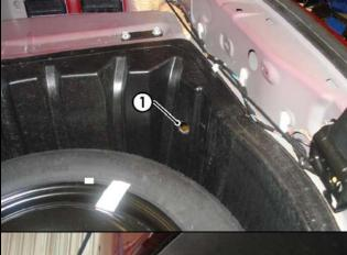
9. From outside of the vehicle, route the Tail Harness (tail length 1800mm) (1) into the bumper towbar cut out (2) and into the spare wheel well via the drilled out hole.
