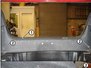
3. Remove the three clips (1) from the RHS luggage compartment trim and then peel open the trim (2).
