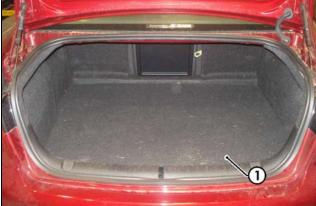
2. Remove the luggage compartment rear trim (1) by removing the cargo strap hooks and the two lower clips (2).
