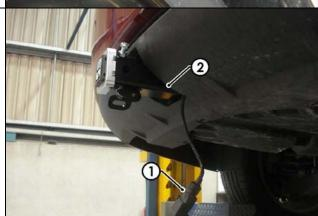
10. Mount the trailer socket (1) on to the towbar socket mounting plate using M4 fasteners (not supplied).
