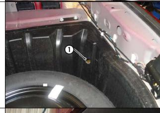
30. From outside of the vehicle, route the Tail Harness (tail length 1800mm) (1) into the bumper towbar cut out (2) and into the spare wheel well via the drilled out hole.
