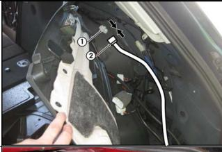
25. Secure the Trailer Patch Harness ground ring terminal (1) using a tech screw (2) as shown.
