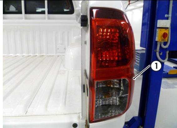
2. From underneath the vehicle, route the trailer patch harness (P/No: 101247-WL) connectors (1) up the RHS tail light cavity.
