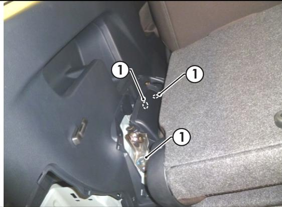
3. Remove the LHS tool access tray and then remove the tools (1).
