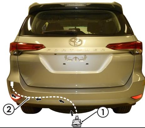
14. Route the trailer patch ORANGE power wire underneath the vehicle following the LHS chassis rail to the engine bay accessory fuse box. Keep harness routing clear of all moving parts, sharp edges or places of extreme heat. Appropriately secure the harness at 200mm intervals using cable ties (not supplied) after routing.
