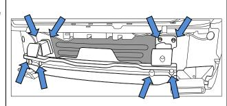
9. Secure towbar to vehicle using 8 x M12 x 1.5 x 45 bolts G10.9, complete with 1 washer per bolt.
