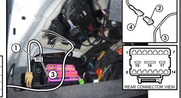
**12.** Secure the trailer patch ground ring terminal (1) to the vehicle grounding location (2) using the existing vehicle fastener.
