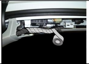
17. Connect the trailer patch connector (1) to the ECU (2). Remove the backing from the back of the ECU and mount the ECU (2) onto the sheet metal area (3). Ensure ECU is mounted with the connector pointing downwards.
