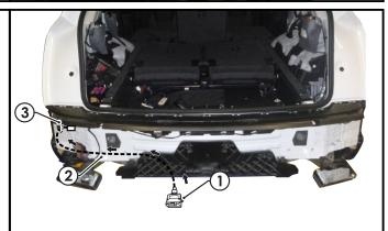
**21.** Connect the tail harness 8-way connector (1) to the trailer patch 8-way mating connector (2).
