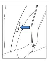
6. Partially remove wheel arch trim and remove 2 x Torx screws securing the bumper to the vehicle.
