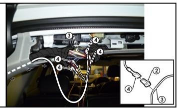
16. Tape up the vehicle harness suitably, ensuring the harnesses inside are not tight and retain enough slack to have free movement when the rear door opens and closes.
