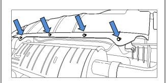
5. Inside wheel arch, remove 1 x nut securing wheel arch TRIM.
