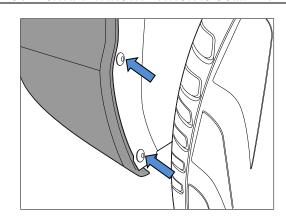
2. In rear wheel arch, lift felt and remove 1 x Torx screw securing bumper.
