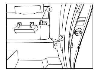
15. From the luggage compartment, remove the 5 push clips (1) securing the LHS trim (2).
