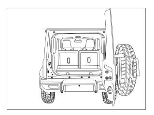
2. Remove 4 x M10 hex screws and 2 x scrivets from topside of bumper.
