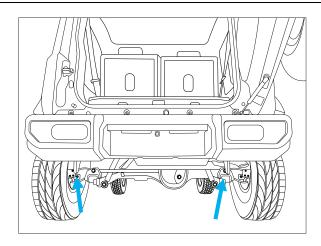
5. Peel away bumper and disconnect wiring on both sides.
