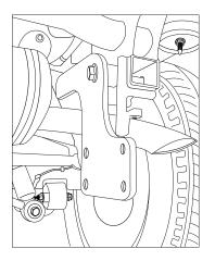
8. Attach towbar central section to each sidearm using 4 x M12 bolts complete with 2 x washers and 1 x nut per bolt.
