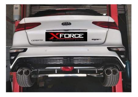
Note: When you first start your vehicle after the installation of your new XFORCE Performance Exhaust System, there may be some smoke and fumes coming from the system. This is a protective oil based coating used in the manufacturing of mandrel bent performance exhaust tubing. This is not a problem and will disappear within a very short period of time after the exhaust has reached normal operating temperatures.
