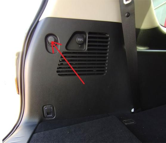
h. Remove the lower tie-down fixture by lifting plastic flap and removing its securing bolt. Repeat on opposite side.
